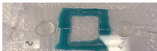
Figure 1. Assembled flow chamber lying coverslip down.
